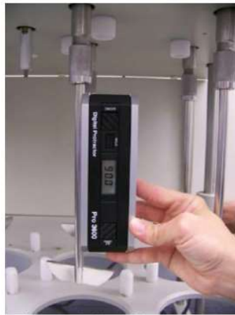
Figure 1. Electronic level giving 0.0° reading on the base plate of a test assembly.
