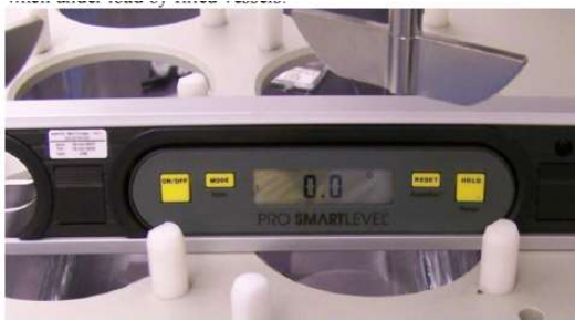
Figure 1. Electronic level giving 0.0° reading on the base plate of a test assembly.
